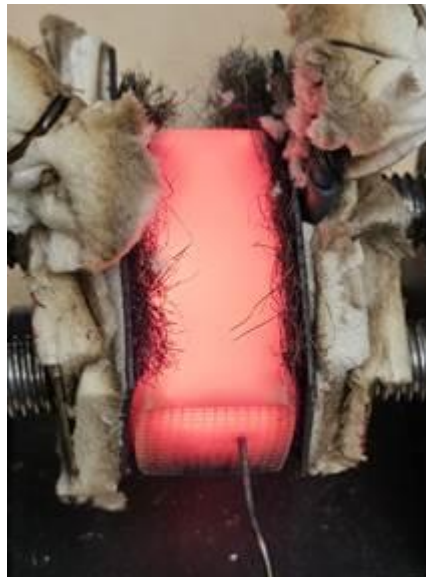
Coated honeycombs with electrodes, fiber mats, and metal housing
