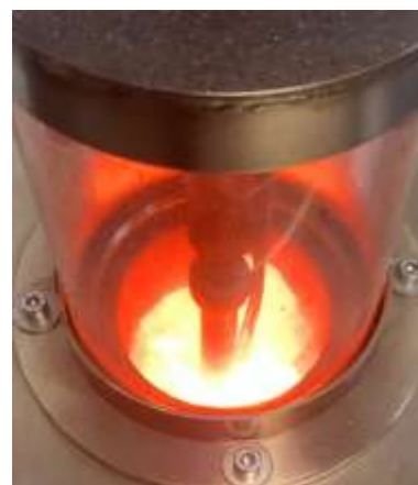
Figure 1. ETFB reactor prototype, operating at 1000 °C
