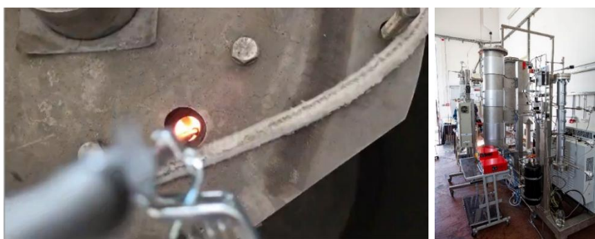
Figure 1 Fluidized-bed material glows at 1000 C in ETFB reactor. Methanol synthesis yielded 2 kg of MeOH on pilot scale.
